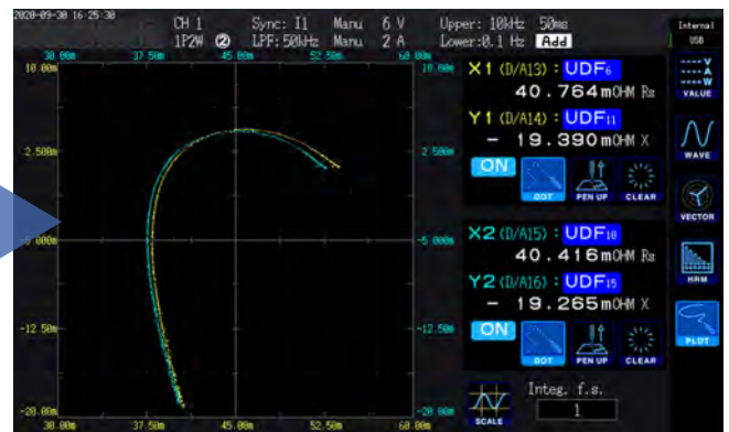
Cole-Cole plot diagram swept up to 10kHz during discharging
