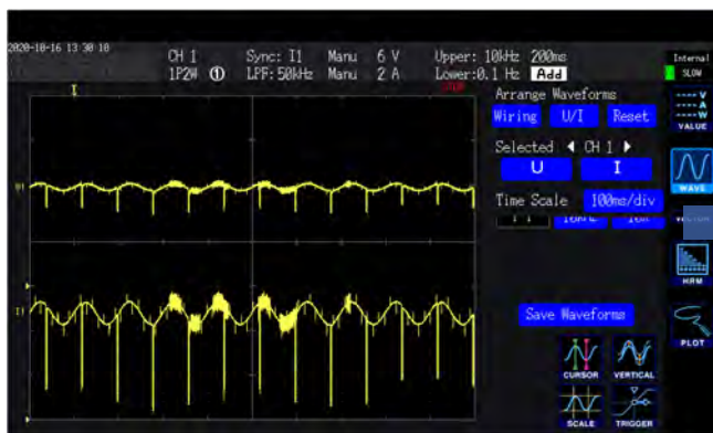
Discharge current and voltage waveform with noise
